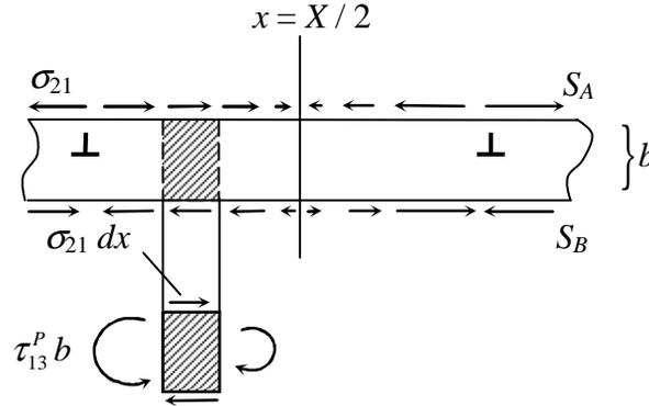
Figure 8. Antisymmetric stress state in the PEIERLS model of an edge dislocation
