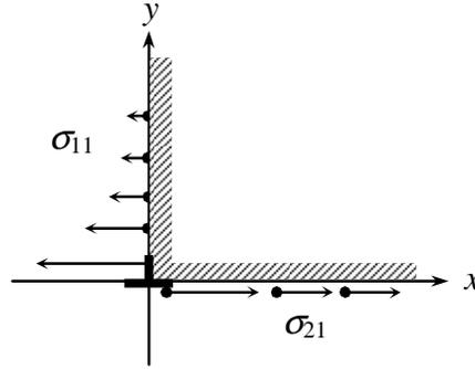
Figure 9. Proving the lack of associated edge stresses at the center of a dislocation.
