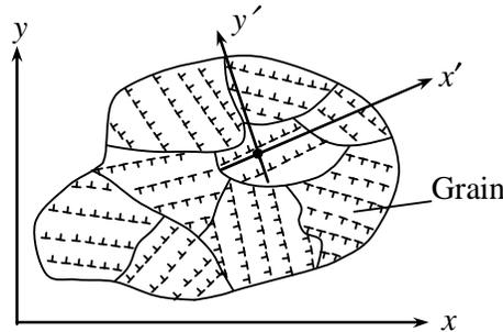
Figure 10. Two-dimensional schema for our polycrystal model.
