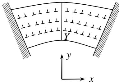
Figure 1. Macroscopically-homogeneous distribution of edge dislocations in a plastically-bent beam (schematic).
