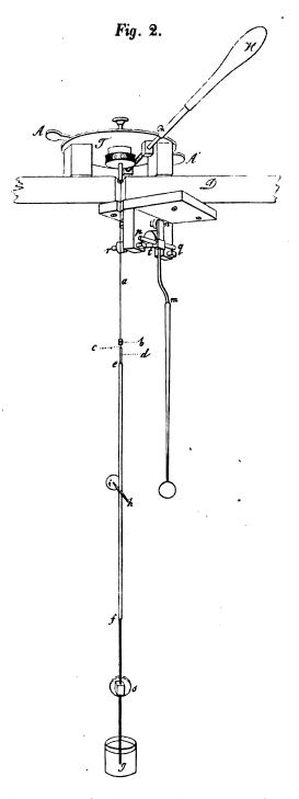
The torsion circle T was fixed over the center of the lid, whose crosssection is denoted by D in Figure 2, whose alidade AA' allowed one to read off the individual minutes from its vernier scale and would lead to a finer
