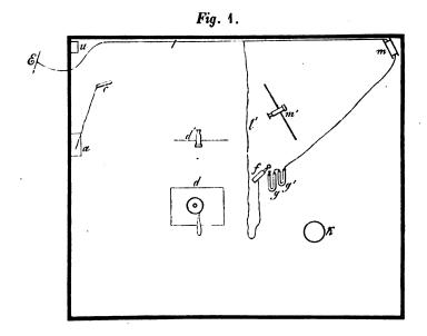
The tangent galvanometer is denoted by m, whose multiplier wire is connected to the Earth at its one end by a conducting wire l that is soldered to a plate E that is buried in wet soil, while the other end of the wire leads through the air to the long U-shaped glass tubes g and g', which are filled with water. m' represents the scale and telescope for observing the needle of the tangent galvanometer, which is provided with a mirror.
